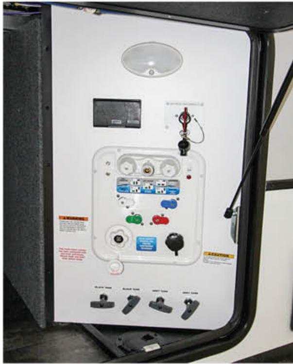
The Alliance Utility Center brings vital connections to one convenient location for management of water hookups, coaxial connections, battery shut off, and tank pulls. Additionally there is a light for when the sun is down, a quick connect sprayer to wash up after dealing with the business end, and a 110V outlet for your convenience.
