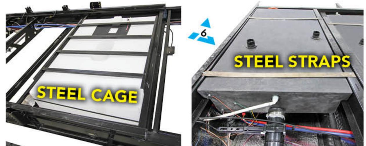
Our fresh tanks are encased in a robust steel cage. Waste tanks are molded to rest on full length steel Z rails and secured with steel straps to prevent shifting in transit.
