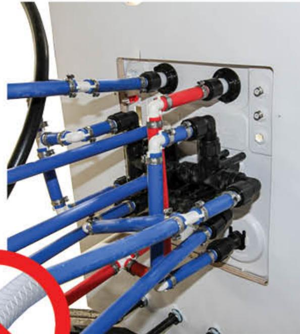
Real PEX water lines are used throughout to create a reliable and temperature resistant plumbing system. Traditional braided lines (commonly used by some manufacturers) provide an inferior fit at the connection points, making them more susceptible to water leaks.
