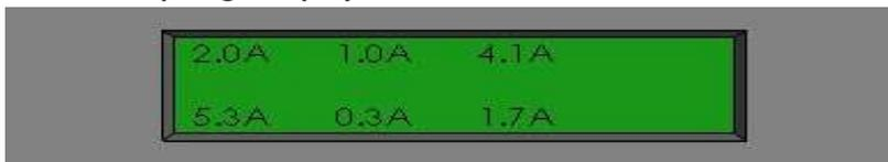
Pressing **Enter** at the **History Menu** shows past power consumption in **Watt hours** per circuit, the first display will show circuits 1 2 3, next display shows circuits 4 5 6, then previous hours as you press the “**Down**” button. Pressing the **Enter** button again returns you to the History Menu screen.
