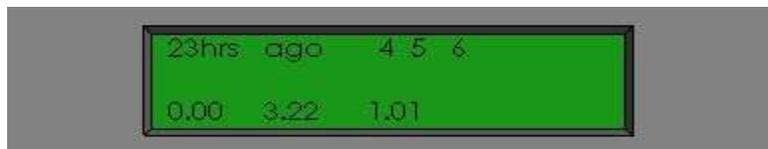
Pressing **Enter** at the **Max Power Setting Display** allows editing of the maximum Amps allowed by the system. Press **Up** or **Down** to set Amps, then **Enter** to save.
