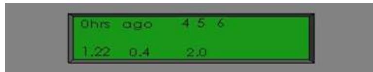
Continue to press **Down** to display 0 hours up to 23 hours for circuits 1, 2, 3, 4, 5, 6
