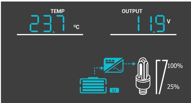
Inverter Temperature Celsius / Output Volts AC
