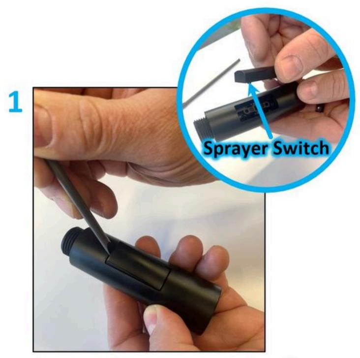
Remove the **sprayer switch** with a flathead screwdriver.
