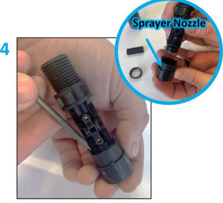
Unclip and remove the **sprayer nozzle** with a flathead screwdriver.
