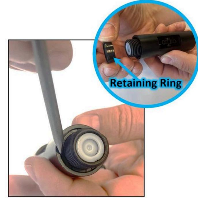
Remove the screw on retaining ring counterclockwise (Use a flathead screwdriver to get it started)
