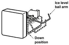
When the ice maker thermostat senses the preset temperature for the ejection of the ice cubes, the fingers will start to rotate, dumping any ice cubes and filling the mold with water. When the storage container is full, the bail arm will come in contact with the ice cubes. The bail arm cannot return to the full down position and the ice production is stopped until the bin is emptied, or ice cubes are removed.
