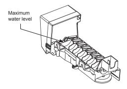
If necessary, change the water flow by adjusting the water supply. For instructions, see ADJUSTING THE SIZE OF CUBES.
