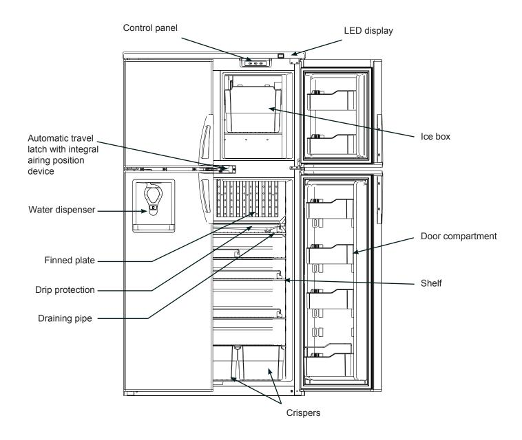
General view of the appliance. Model shown is equipped with ice maker and water dispenser. Appearances and features may vary depending on model. Quantity and position of items may also vary.
