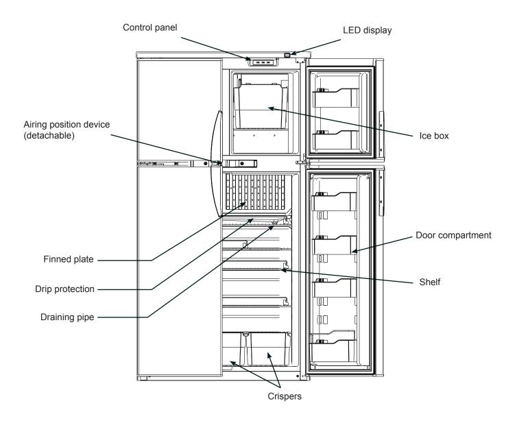
General view of the appliance. Model shown is equipped with ice maker. Appearances and features may vary depending on model. Quantity and position of items may also vary.
