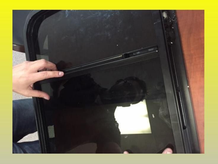
8.) Slide track back into window frame around the glass
