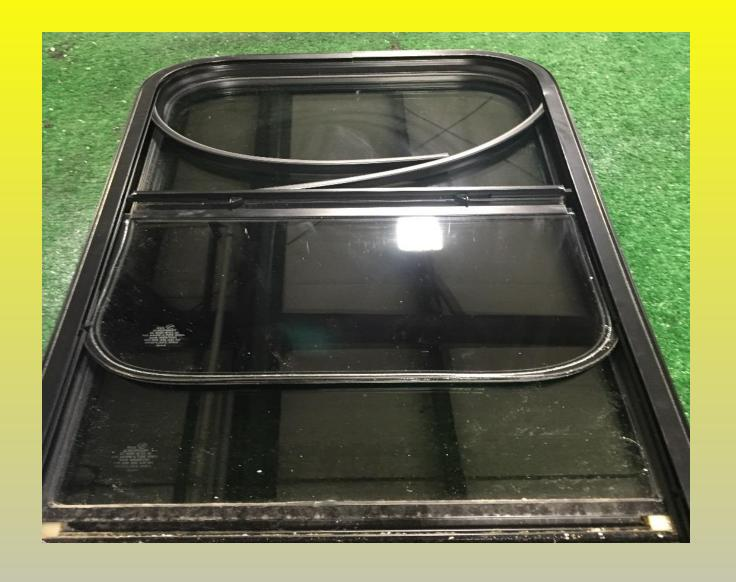
4.) Push latch plungers in and remove sash from window frame
