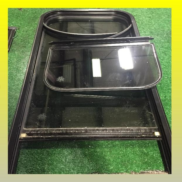
5.) Remove latch screws located on the back of the window sash and slide out
