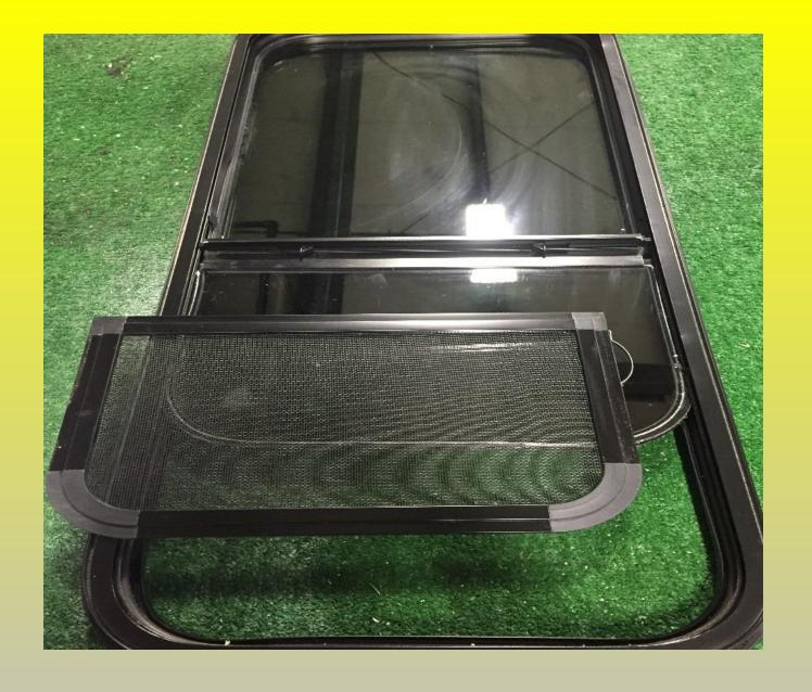
3.) Push both latches in simultaneously and gently remove window sash
