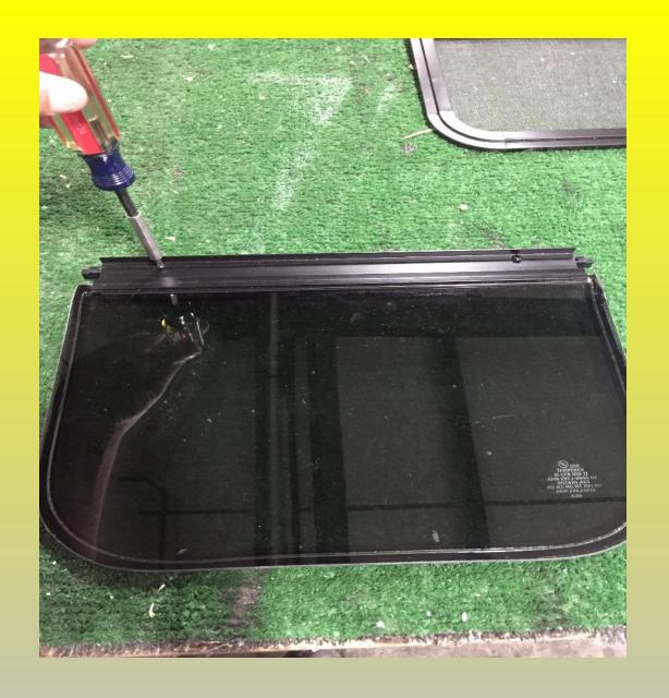
6.) Insert replacement latch and reinsert set screw
