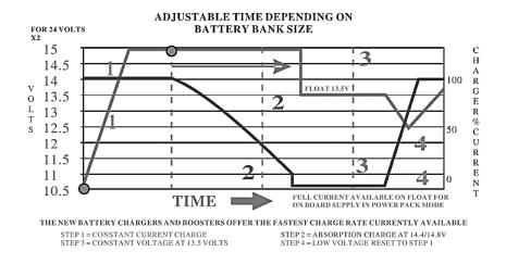
**Bulk Stage:** The charger will supply constant current until the battery voltage reaches the boost voltage. The software will calculate the time charging began up until the battery voltage reaches 0.3V below the boost voltage. It uses this time to as T0 and T0×10 = T1.
