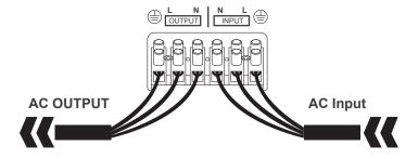
The AC input must never be connected to the AC output as irreversible overload or damage may result
