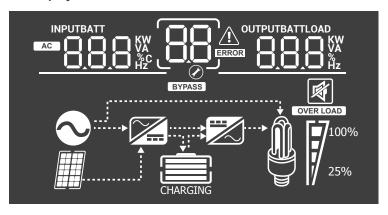
NOTE some PCL inverter-chargers will differ in the LCD display on erroneous icons that do not influence or modify the working mode of the inverter-charger.
