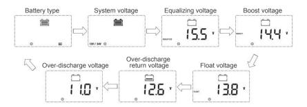
To enter the programming interface simply press and hold the right arrow button. After entering this feature press the Enter/Right button to switch between parameters. To change the parameters, press the Up or Down button. To save the parameter press and hold the Enter/Right button.
