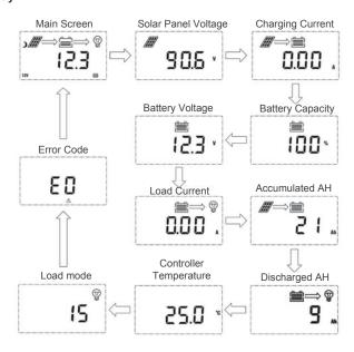
The Battery Capacity (SOC%) is estimated based on the charging voltage.
