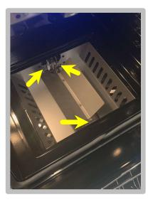
Loosen 3 screws as noted above and remove bottom burner tube.
