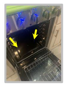
Loosen the two screws as noted above and remove bottom plate inside oven.
