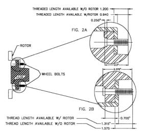
Fig 2. Typical 6000 lb. axle & below
